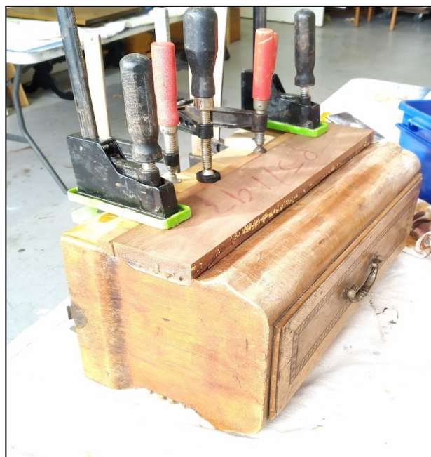
Martin Lawtons "jig" to fix the veneer to the cover
