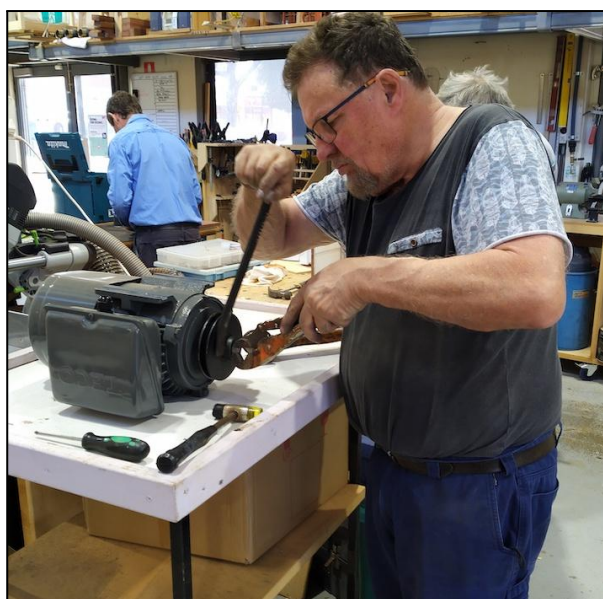
Bill Barton fitting the modified pulley to the new motor
