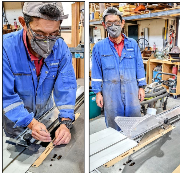
Shoichi Nakanishi fitting the zero tolerance insert plate
