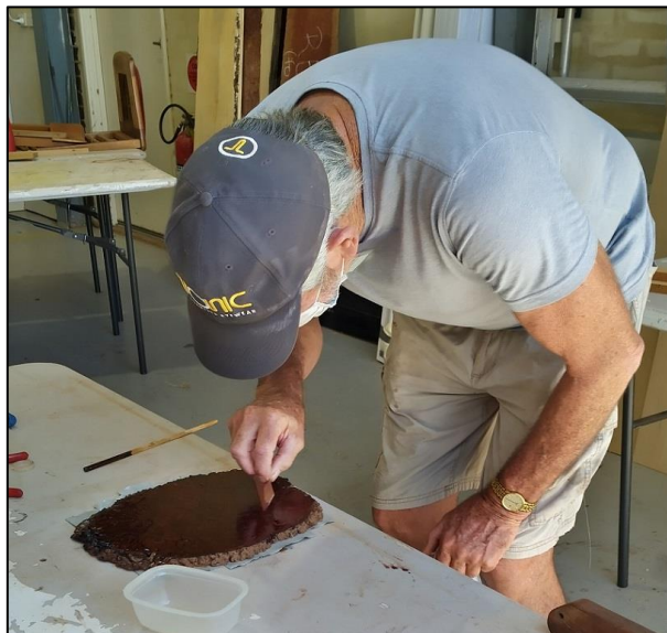
Ken McCracken filling the voids with resin
