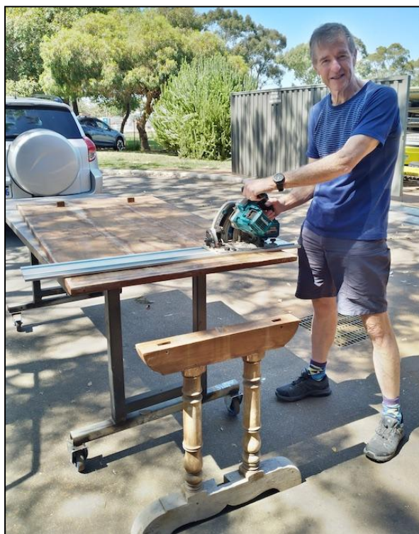
Bob Creelman trimming the table top with the Track Saw
