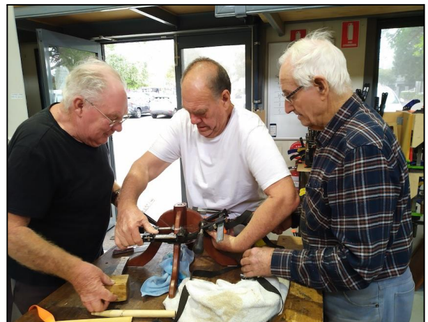
Martin Lawton (left) holds the legs while Mike Harrison (centre) adjusts the clamps on the legs and Peter Repton tightens the strap clamp
