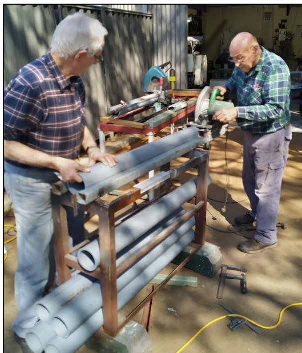
Peter Repton (left) and James Turner setting up the first jig to cut the pipes into two semi- circular pieces. The second jig to cut the individual houses is in the background
