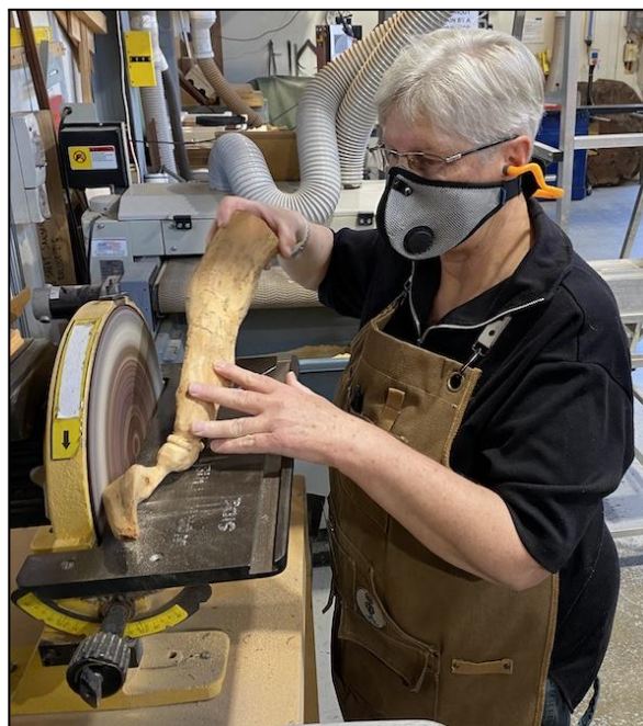
Jan Lucas sanding and shaping the piece of Huon pine
