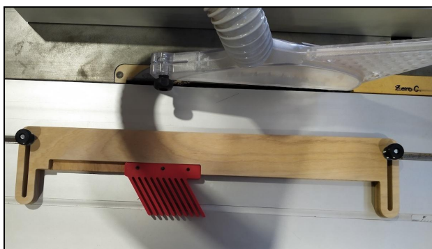
Shoichi Nakanishi's Featherboard for the Panel Saw
