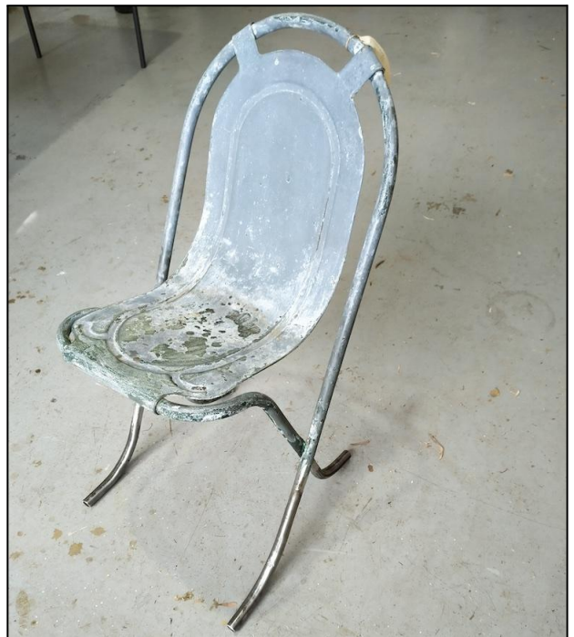
Metal Chair showing the three legs repaired by Peter Repton
